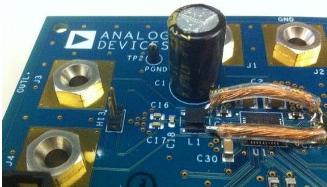
Figure 3. Board Modifications for Mono Mode
